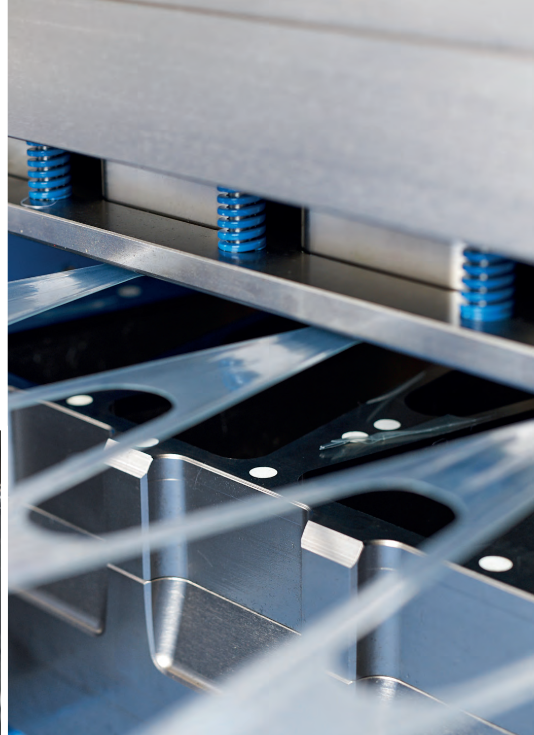
complete cut punch for individual packaging shapes
